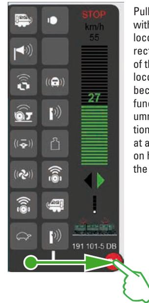
Pull the red circle with a small white locomotive in the direction of the center of the screen: The locomotive functions become visible, eight functions per column. Up to 32 functions can be shown at a time depending on how far you pull the list up.
