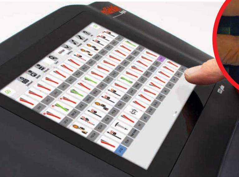
**Dragging and Zooming:** Thanks to the high-resolution Touchscreen, simple touches are all you need to operate this device – such as with a Smartphone or a Tablet. For example, in order to enlarge the track diagram, you drag with the thumb and index finger „away from each other“.
