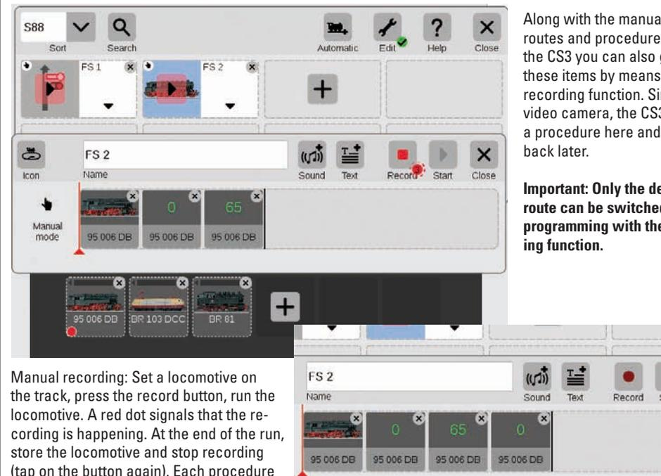
Along with the manual entry of routes and procedures, with the CS3 you can also gather these items by means of a recording function. Similar to a video camera, the CS3 records a procedure here and plays it back later.
