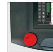
Tap on the speed controller and the green bar becomes visible: The locomotive runs. Alternatively wipe over the bar or control with the red control knob – even if the locomotive controller is faded out. You change the direction of travel with the green arrow – or by pressing on the control knob.
