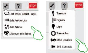
All kinds of items can be added by means of this option: Tap on the tool symbol for the item list and select „Add Article“ in the drop-down menu (left image) as well as in the extension „Misc Devices“.
