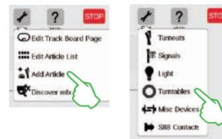
A turntable is also easily put into the item list: A drop-down menu opens with a tap of your finger on the tool symbol for the item list („Edit“). Here you select „Add Article“ (left image). Tap on „Turntables“ in the menu that follows.
