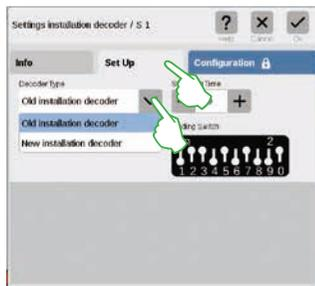
You can do other settings in the tab „Set Up“. Here you select the type of decoder and you can also change the switching duration.
