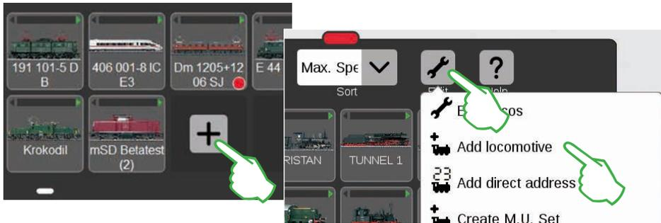
Locomotives without an mfx decoder are added by hand. To do this simply tap on the large plus sign at the end of the locomotive list. You can also tap on the tool symbol („Edit“) in the locomotive list and select „Add locomotive“ in the menu that is turned on.
