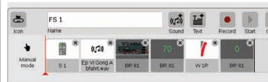
The route can be assembled step-by-step by means of drag & drop. Each individual point (speed, signal and turnout settings, etc.) can be adjusted individually in the process (see the following pages).
