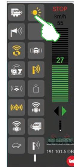
The functions are switched by tapping on the function symbols. For example, in the image to the left the light, coupling/uncoupling, the whistle, and the blowers are being activated.
