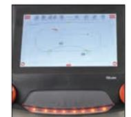
When the speed bar is shown in red, the Stop mode is activated. Press the Stop button or tap on the Stop symbol on the upper corner of the locomotive controller in order to turn it off.
