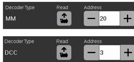
On the lower edge of the „Info“ tab for the locomotive settings, you will find the option „Read“ for MM and DCC locomotives: Tap on it and the CS3 takes over the address set in the locomotive decoder.
