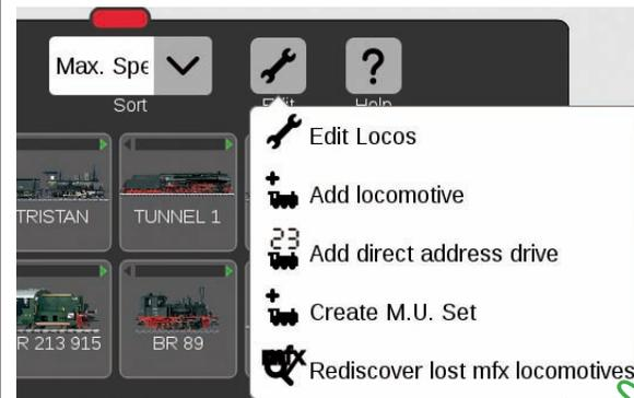
In rare cases, it can happen that an mfx locomotive is no longer displayed in the locomotive list. This option can be helpful. All of the existing data are checked and the system investigates for missing mfx locomotives.
