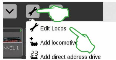
You activate the editing mode with a tap of your finger on the tool symbol and then on „Edit Locos“ (left image). You will recognize it by the green check mark appearing at the foot of the tool symbol (image below): All of the locomotives now appear with a dashed frame and they can be deleted by means of a brief touch on the „X“.
