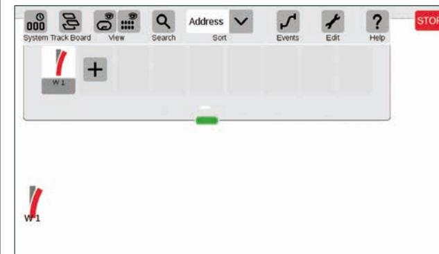
**Important:** The CS3 automatically drops every newly added item on that board that is active at the time the item is being added. Therefore, make sure which board is in the foreground.
