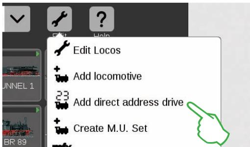
Tap in the locomotive list on the tool symbol („Edit“) in order to control and run a locomotive directly by means of its address and then select the „Add direct address drive“ (left image) in the drop-down menu that opens.
