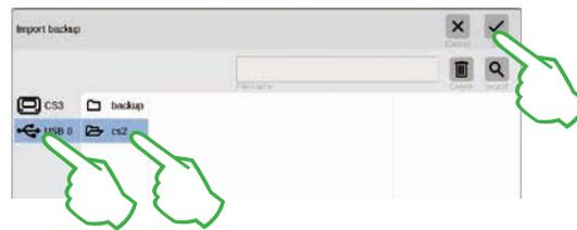
In the file selection dialog, tap on „USB“ and on the directory containing the CS2 backup. Select the backup and confirm with „Ok“. After a few moments, you will receive the start screen for the CS3.
